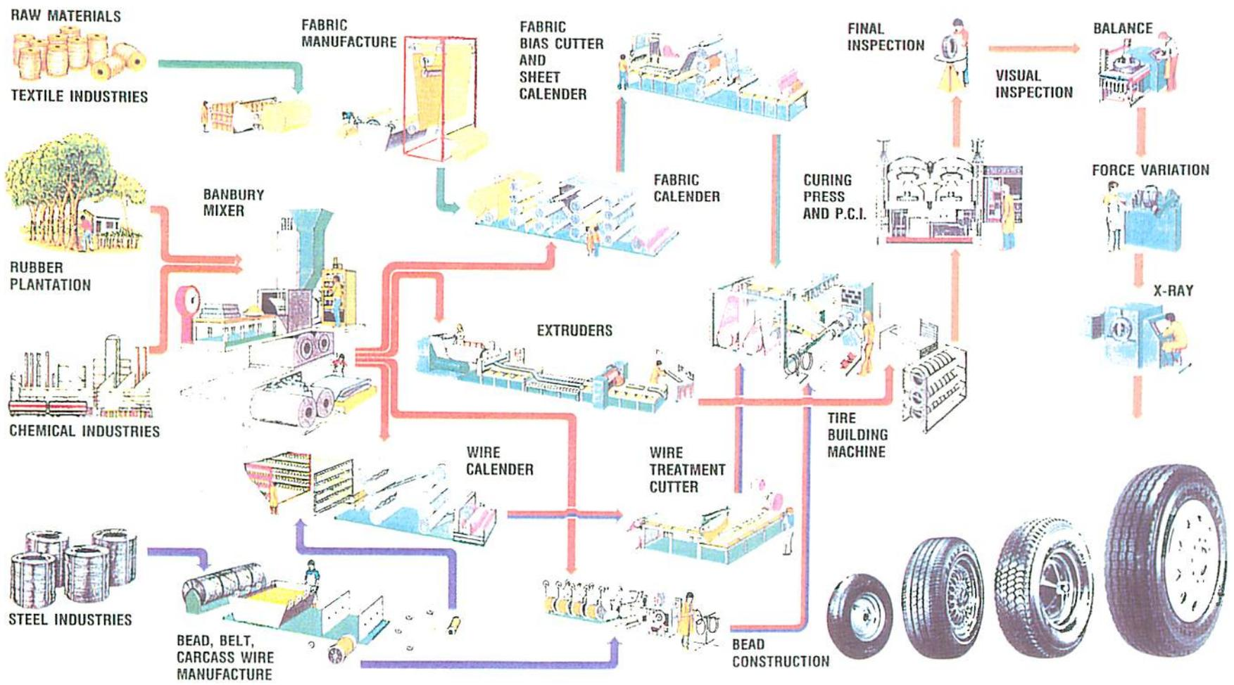
FIGURE 23 The tire manufacturing process.
